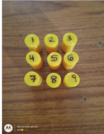
Figure 5: Compression Specimen Prepared from 3D Printer
