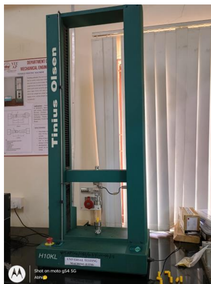
Figure 6: Compression Specimen Placed in UTM
